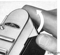
One full movement of the lever tensions the shutter, and advances the film and the film counter. A spring then returns the lever to its original position.
