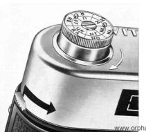
After the last frame the exposed film must be rewound from the take-up spool into the daylight cassette:
