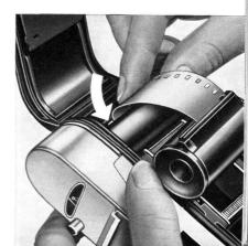
Before closing, the loaded camera must appear as shown in the illustration on the right. The film lies flat in the film track, with the teeth of the transport sprocket engaging the film perforations.
